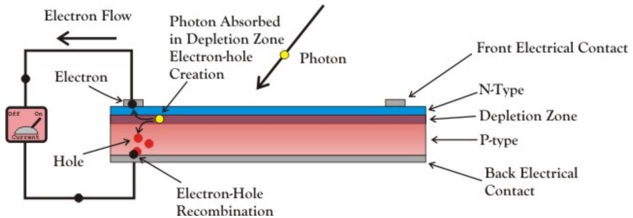
So how well does this all work? That depends on what you want to do. Solar cells can directly provide electrical current, which in turn can pass through some load (motor, toaster, cell phone charger) and do work. Electrical power,  $P$ , is a measure of the energy output per time. It can easily be measured in electrical circuits as it is equal to the current( $I$ ) multiplied by voltage( $V$ ) of the circuit.
