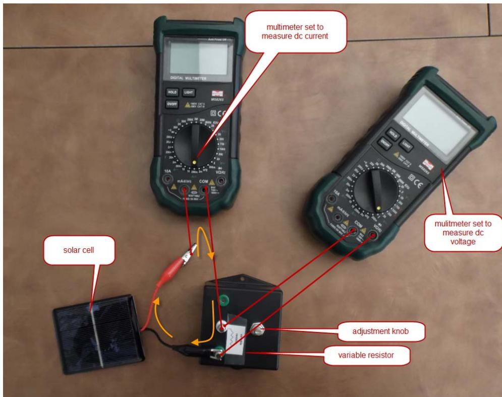
The orange arrows show the direction of current flow. To measure current, one multimeter is in series (current flows through it) and to measure voltage, the other multimeter is in parallel (no current flows into it).
