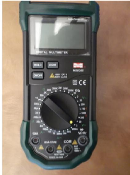
The multimeter can measure current, voltage, resistance, and many other things depending on its settings. Its function is controlled using the large dial, and it matters which input ports are used. You always attach one probe to the COM port, and depending on what else you want to measure the other probe to another port. Wire colours don't matter. If you attach something incorrectly, the multimeter beeps at you.
